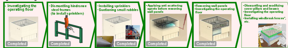
Flow of building cover dismantling
