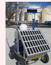
Installation of Dose-rate monitor
