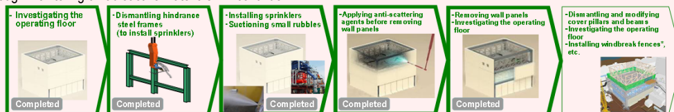
Flow of building cover dismantling
