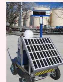
Installation of Dose-rate monitor
