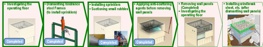
Flow of building cover dismantling
