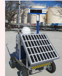
Installation of Dose-rate monitor
