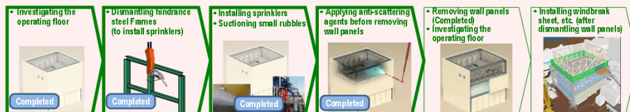
Flow of building cover dismantling
