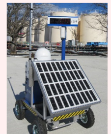
Installation of Dose-rate monitor
