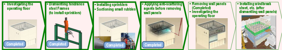
Flow of building cover dismantling
