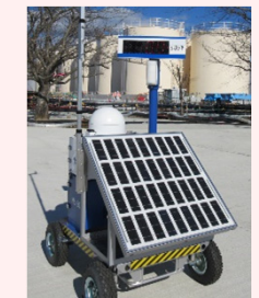
Installation of Dose-rate monitor
