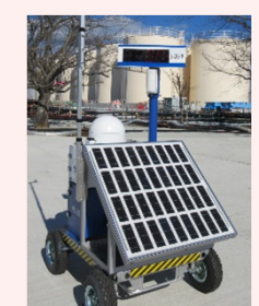
Installation of Dose-rate monitor
