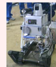
Robot for investigating the contamination status (gamma camera mounted)
