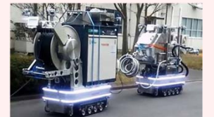
Dry ice blast decontamination equipment
