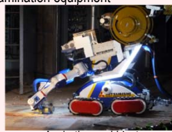
Aspiration and blast decontamination equipment
