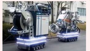
Dry ice blast decontamination equipment
