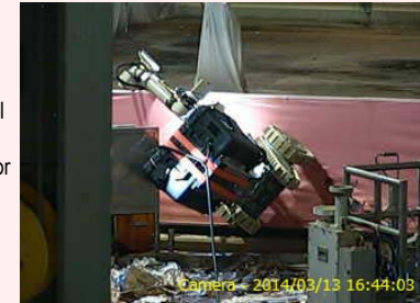
Status of remote-control robot falling down
