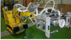
High-pressure water decontamination equipment
