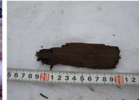
Piece of wood found in the fourth stage impeller
