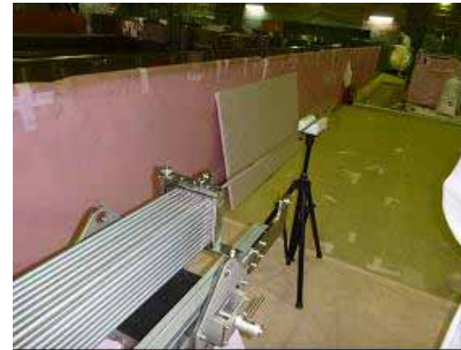
2. Removing a tie rod from the fuel assembly
