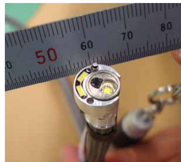
The head of borescope
