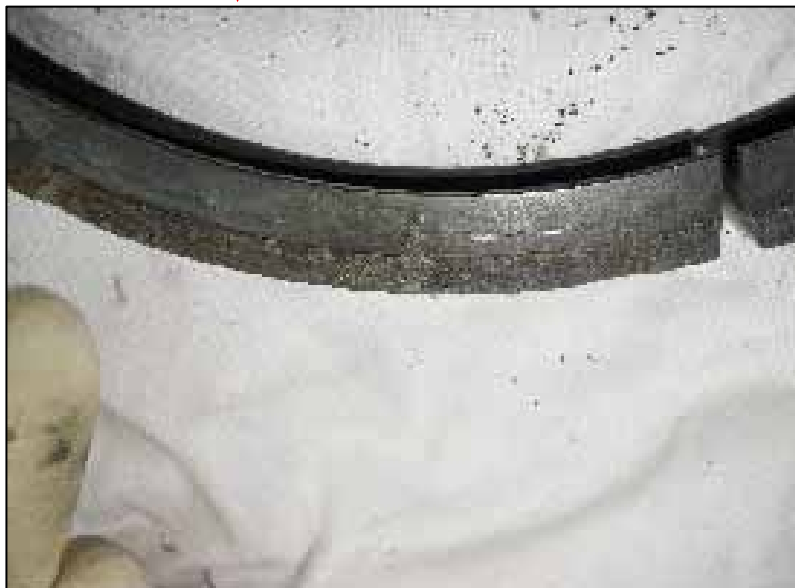
The part of the most remarkable damaged mark hit by the gear
