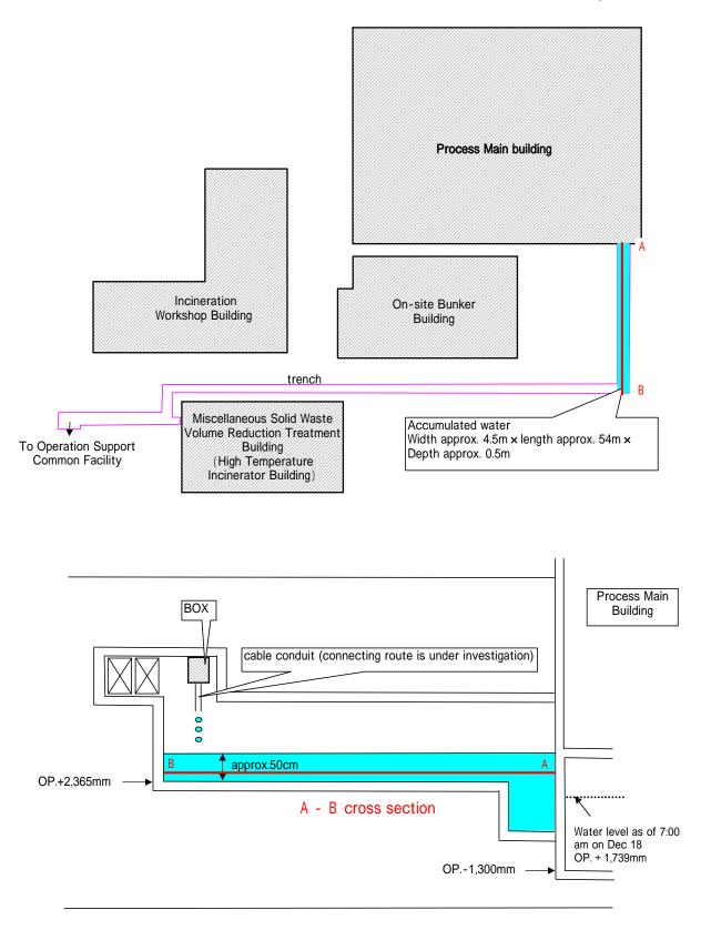
Overview of the accumulated water in the trench between process main building of Centralized Radiation Waste Treatment Facility and Miscellaneous Solid Waste Volume Reduction Treatment Building (High Temperature Incinerator Building)
