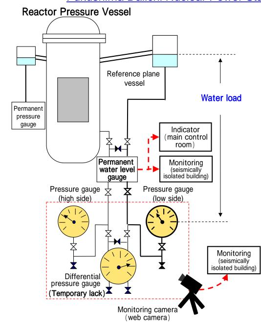
Install a temporary lack (differential pressure gauge and pressure gauge in the dotted line) to the permanent pressure gauge and fill water. Monitoring and confirmation of the indicated value of the differential pressure gauge and the pressure gauge will be implemented afterwards.
