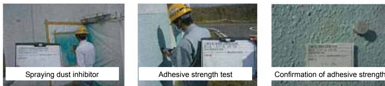
Figure 6: Spraying to the test materials and adhesive strength tests (outer wall (paint finish))
