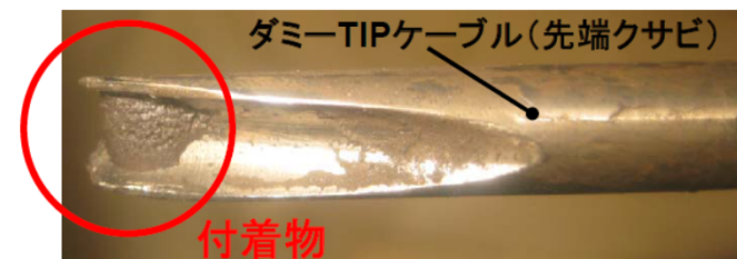
Unit 2 obstruction in the TIP tube
