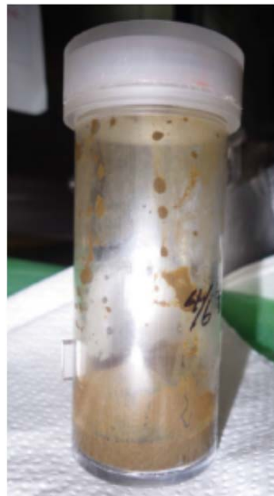
Unit 1 deposit at the PCV bottom
