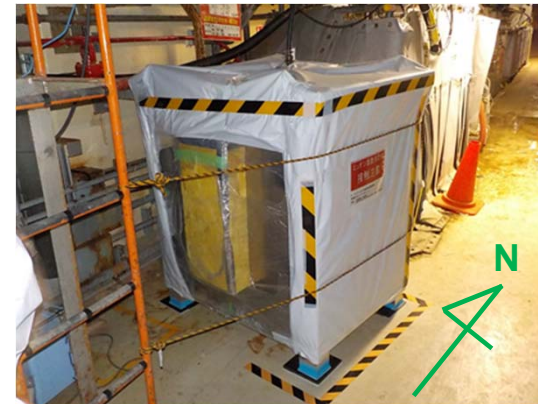
Installation of muon measuring device (small-sized unit, approx.1m × 1m × 1.3m(height))
