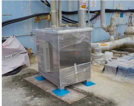
Small-sized muon measurement device*1 in Unit 2 (approx. 1m×1m×1.3m(height))
