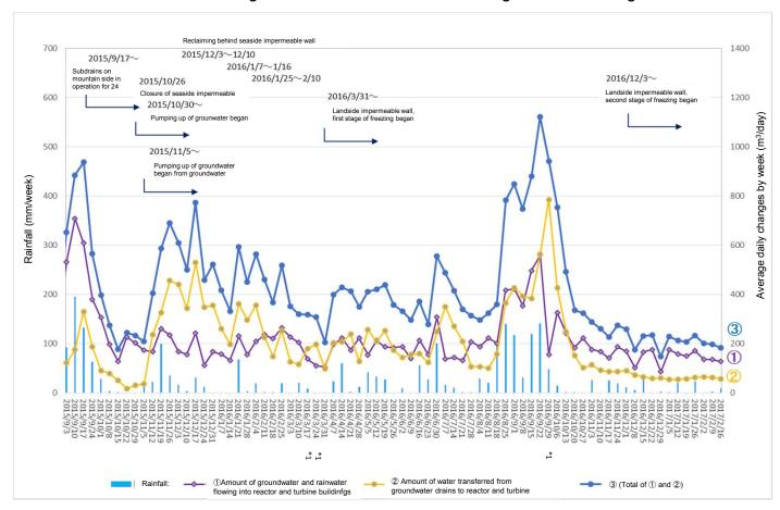
Amount of water transferred from groundwater drains to reactor and turbine buildings (From February 9, 2017 to February 15, 2017/ 24 hours per day)
