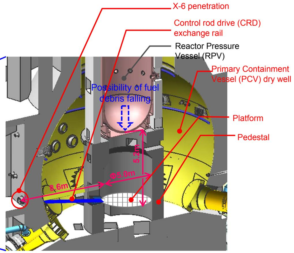
Cross section of the bottom of Primary Containment Vessel
