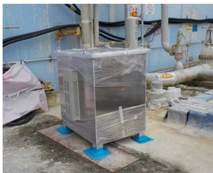
Installation of muon measurement device (small-sized unit, approx. 1m x 1m x 1.3m (height))
