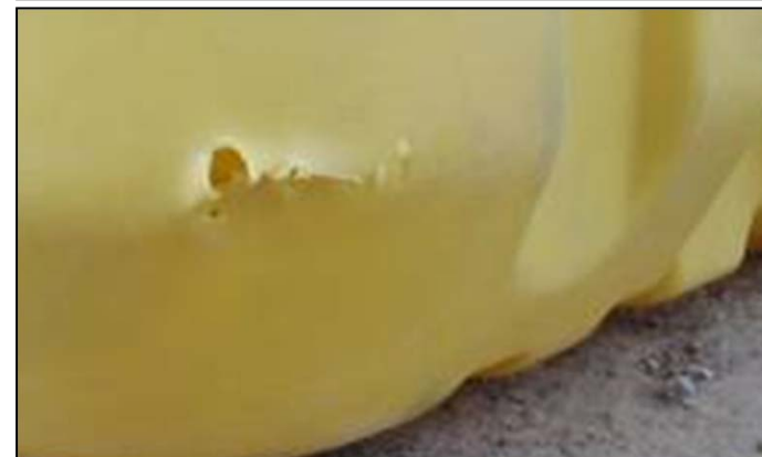
Immediately above: Reproduction test status Upper right: Damage of the leaked tank in the H5 area Lower right: Damage of the tank in the reproduction test
