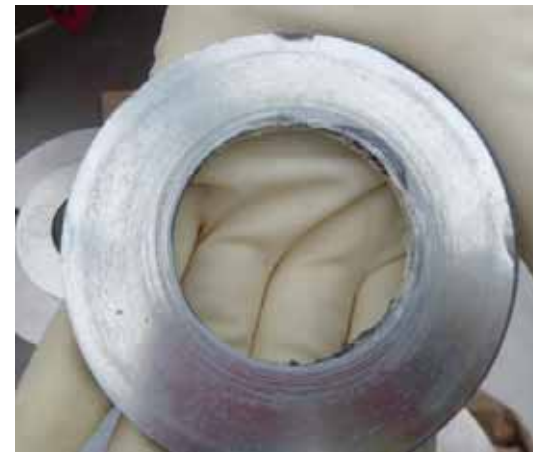
⑫ Treatment column vent pipe gasket-type sacrificial positive electrode
