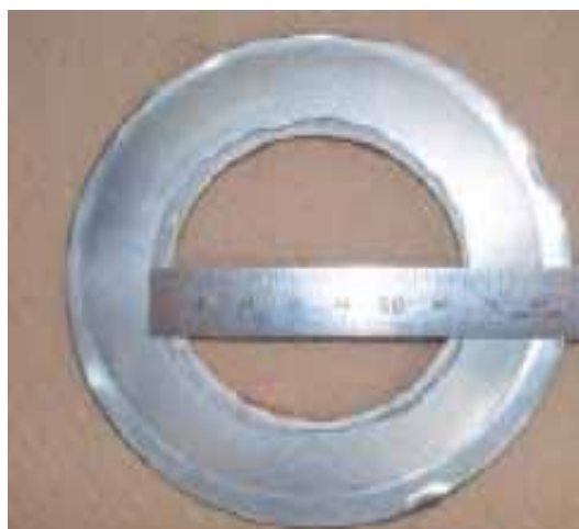
② Slurry transfer pump outlet pipe gasket-type sacrificial positive electrode
