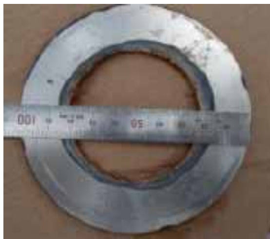
⑦ Supply pump 1 outlet pipe Gasket-type sacrificial positive electrode
