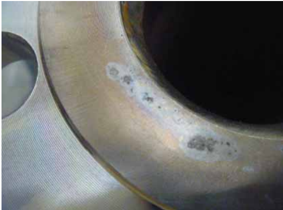
Slurry transfer pump outlet pipe (enlarged) with crevice corrosion on flange-sheet surface
