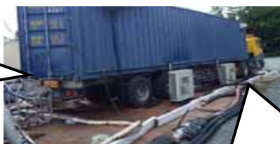
Appearance of RO Unit (vehicle-mount type)
