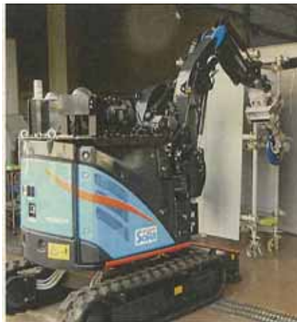
Remote-controlled heavy equipment ASTACO-SoRa
