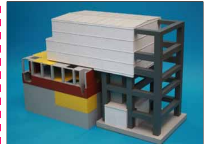
Simulated image of the cover to be installed for fuel removal
