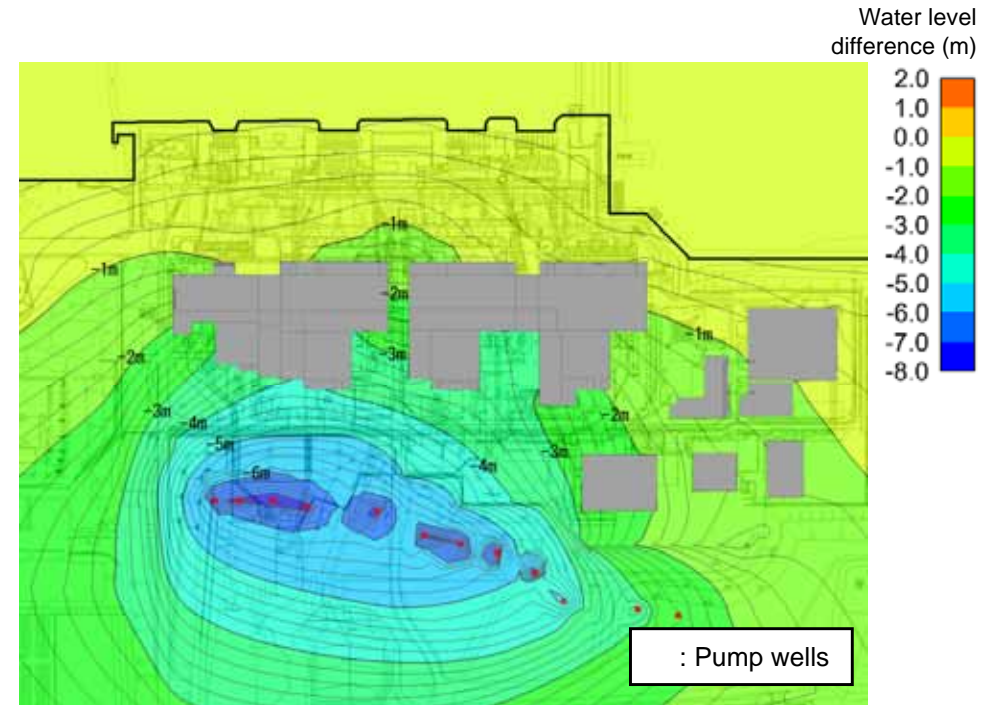
Decrease in the groundwater levels around the buildings (Comparison between before and after the operational commencement of the groundwater bypass)
