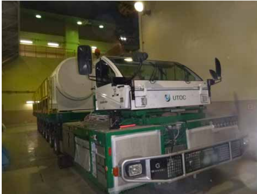
Cask being carried out of the Common Pool Building
