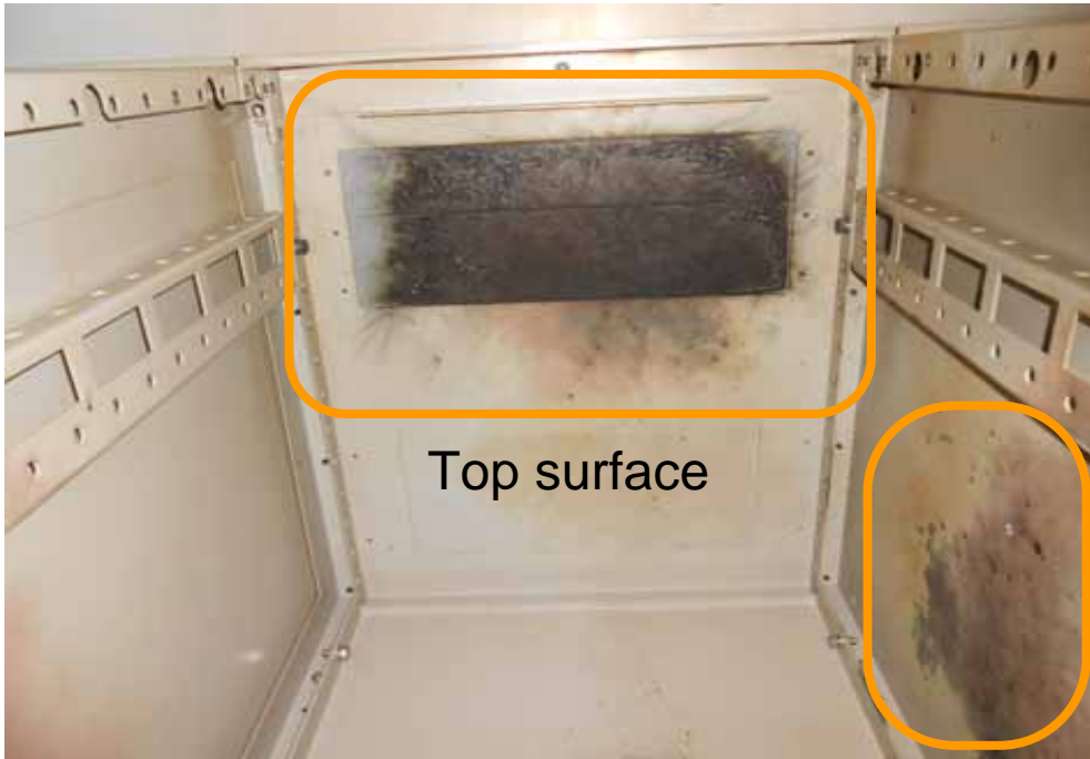
Trace of an arc found on the top surface of unit 5A
