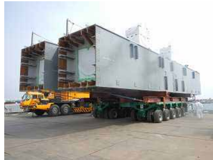
Photo: Transportation of steel members in the power station site (transported via special transportation vehicles)
