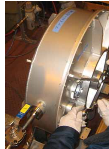
Appearance of the feeding/winding unit for the fiberscope
