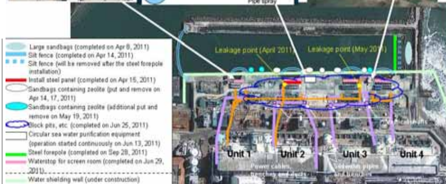
Reinforcement to Prevent Scattering Liquid Containing Radioactive Materials
