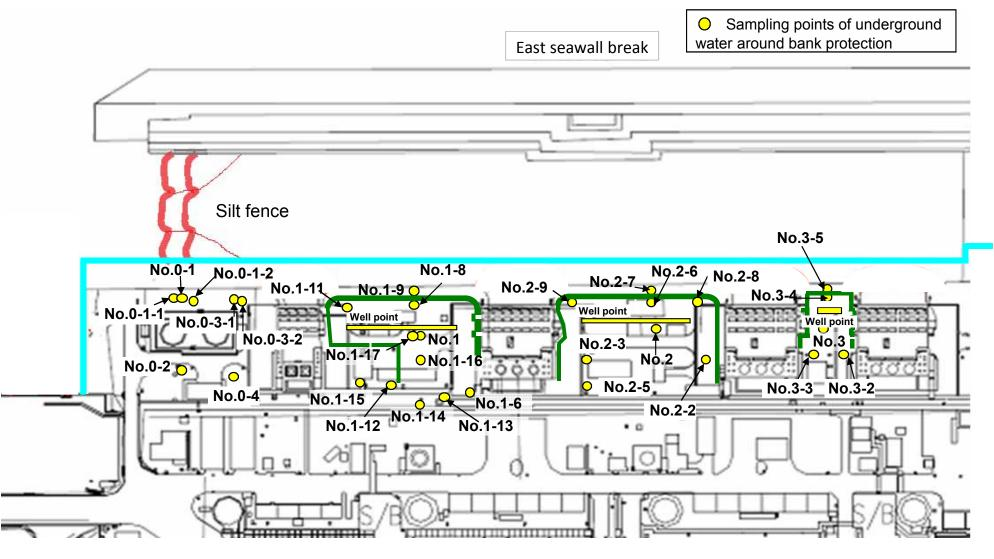
\*Seaside impermeable wall \*Seaside impermeable wall was completed on October 26, 2015. : Location where ground improvement construction was completed, or being implemented (As of April 18, 2014)
