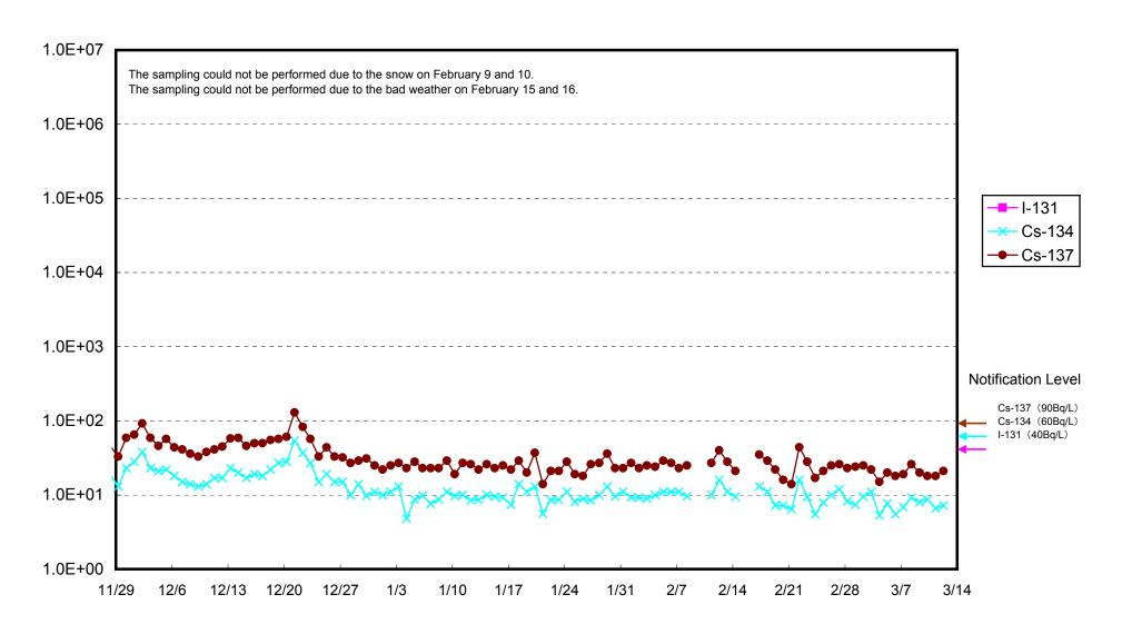
Radioactivity Density of the Seawater at the South of Unit 1-4 Water Intake of Fukushima Daiichi NPS (Bq/L)
