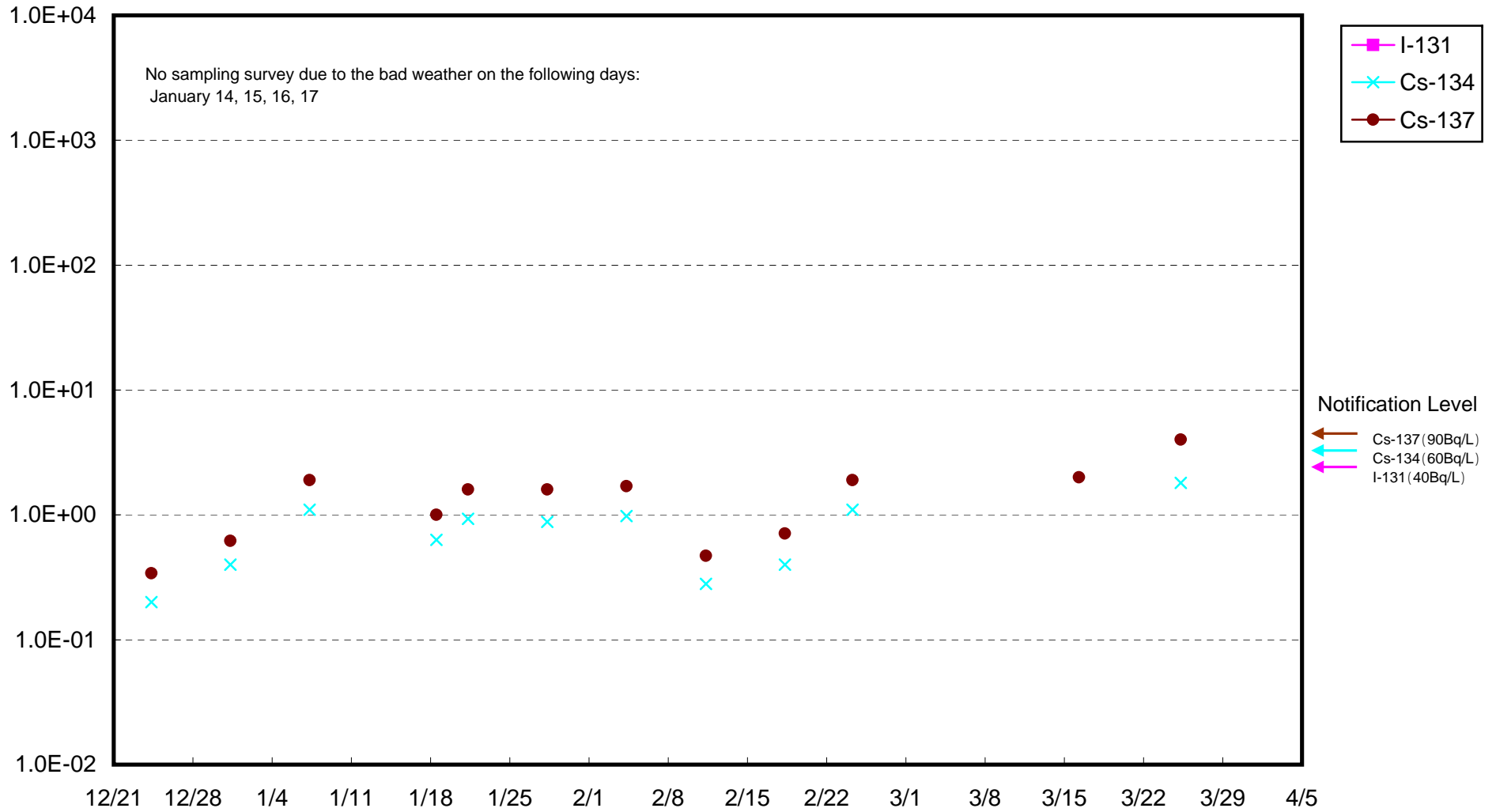
Radioactivity Density of the Seawater at 1F Units 5-6 North Discharge Channel (Bq/L)
