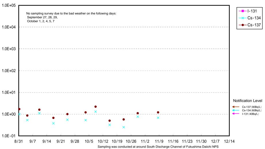
Sampling was conducted at around South Discharge Channel of Fukushima Daiichi NPS (appox. 330m south of Units 1-4 Discharge Channel) until November 25, 2012.
