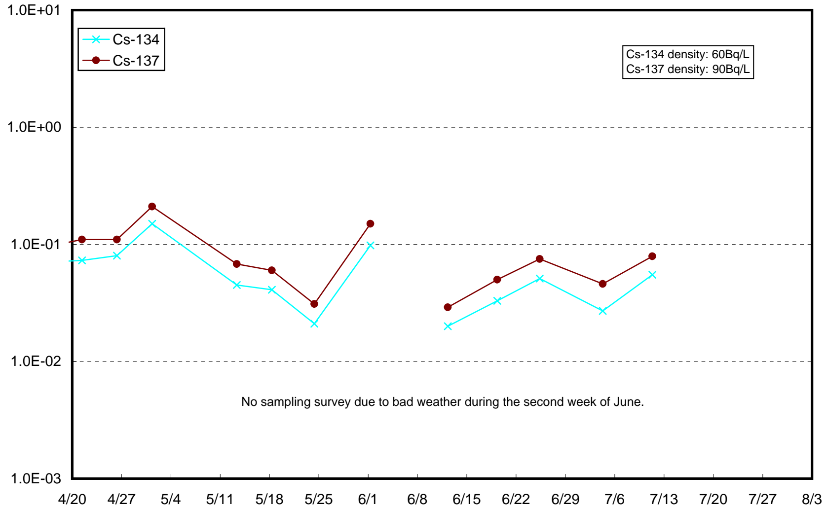
Radioactivity Density of the Seawater at 3km Offshore of Fukushima Daini NPS (T-D9) Upper Layer (Bq/L)
