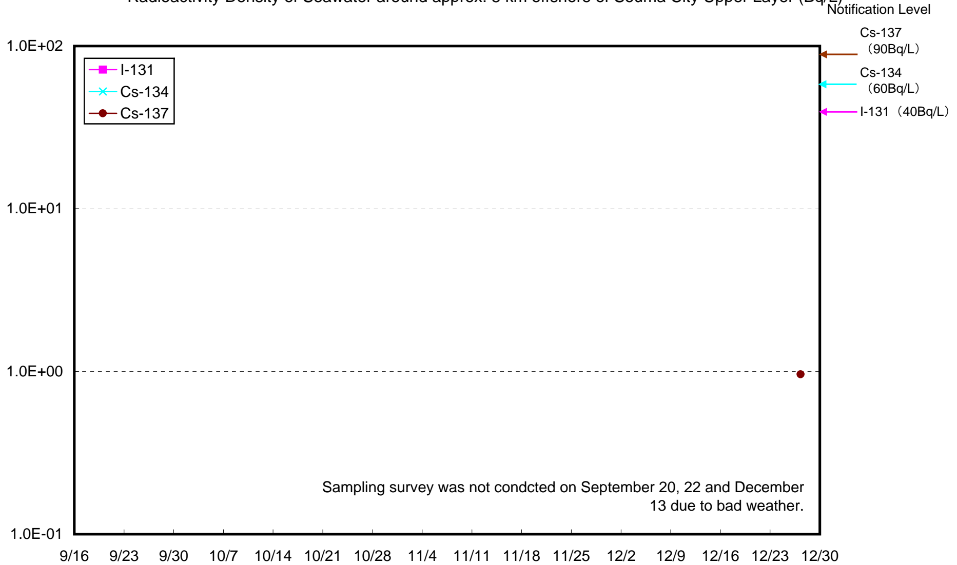
Radioactivity Density of Seawater around approx. 5 km offshore of Souma City Upper Layer (Bq/L)
