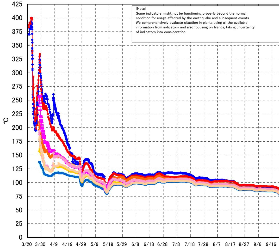
Continuously measured temperatures of feedwater nozzle, N48, and safety valve (exhaust air), 203-4A, have been rising since March 27. In order to compare them with other similar points, some measurement points have been added since 12:30 of March 28.
