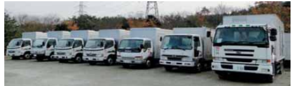
14 Power Supply Vehicles (500-750kVA) and 2 On-board Gas Turbine Generators (4500kVA)
