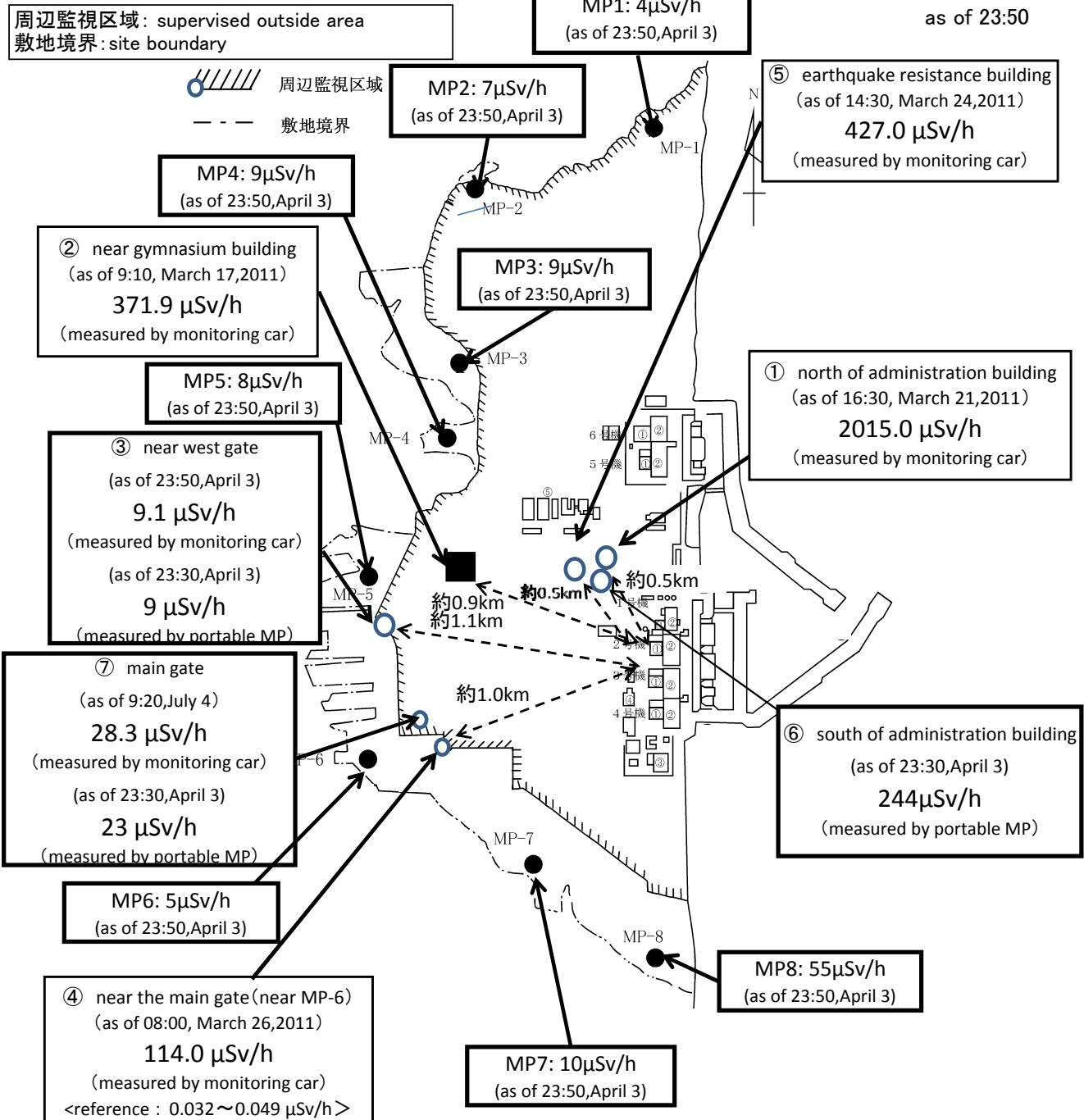
※Reference data indicate the normal fluctuation range of airborne radiation rate.
