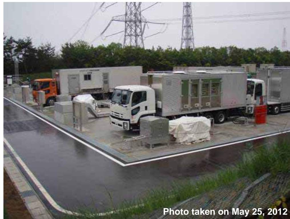
2 air-cooled gas turbine power supply cars have been deployed
