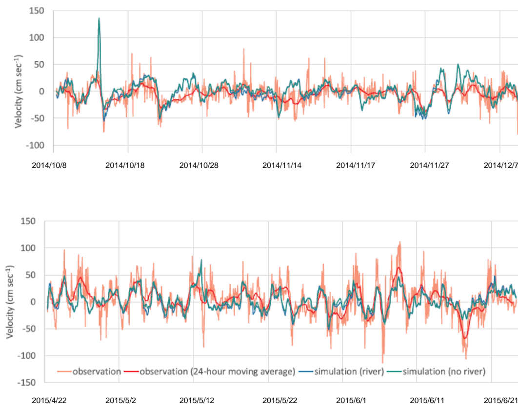
Figure VII-1 Comparison between the flow rate measured near the Fukushima Daiichi Nuclear Power Station and the reproduction calculation by simulation
