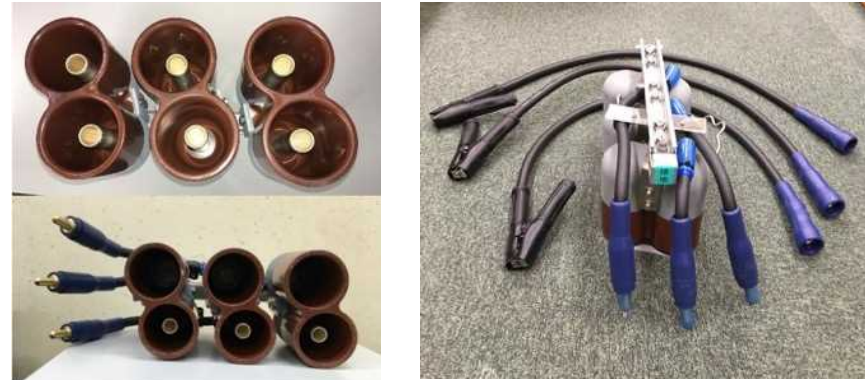
Top: Currently used tool (Closed-circuit kit) Full view of modified tool (earthing kit) Bottom: Modified tool (earthing kit)
