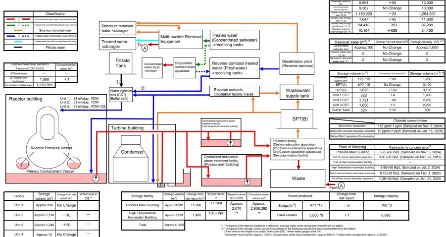
Main operations that have been conducted during the period from February 13, 2025 to February 20, 2025] Water transfer from the Units 1-4 to the buildings (Units 1-4, Centralized radioactive waste treatment facilities) and to the treatment facilities was
