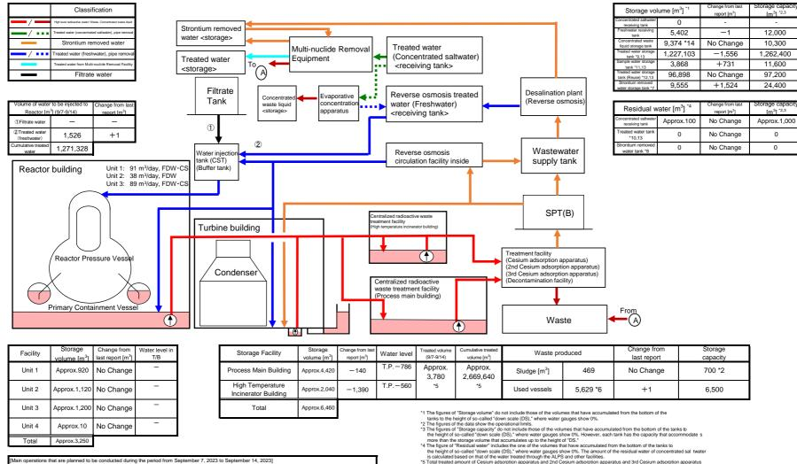
Water transfer from the Units 1-4 to the buildings (Units 1-4, Centralized radioactive waste treatment facilities) and to the treatment facilities will be conducted whenever necessary
