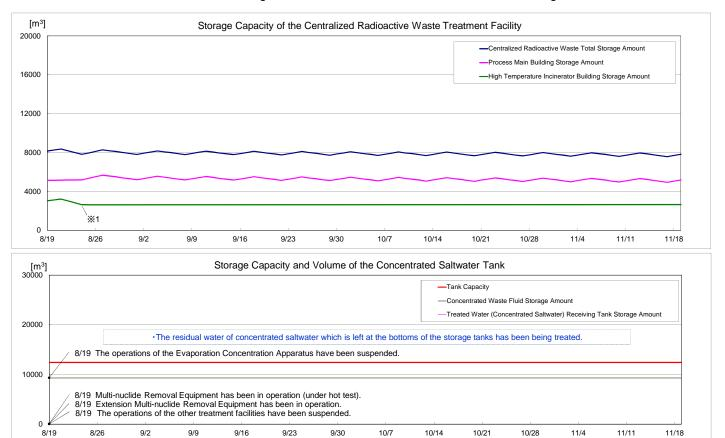
\*1 Storage place of water transported from the Units 1-4 will be changed over from the high temperature incinerator building to the process main building
