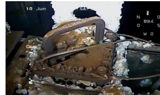
Photo of the top of the fuel repaired with a wire
