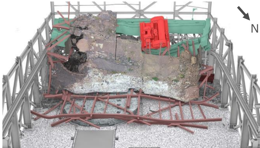
STEP7: Roof frame removal (entire)
